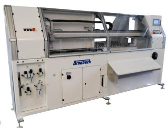
By a tube separator each single core is positioned in a prism. Each single core is fed automatically onto the cutting mandrel.
